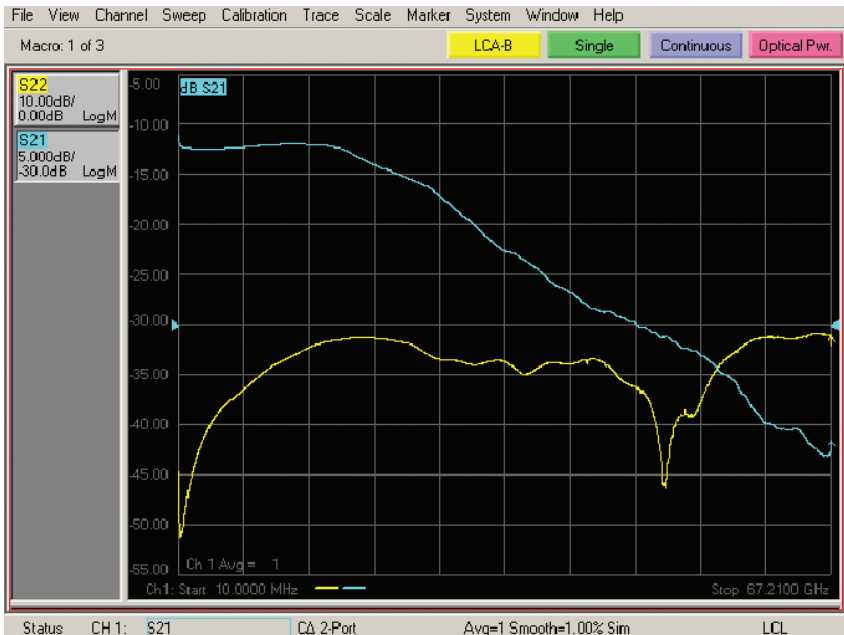
Figure 17. O/E responsivity and electrical return loss measurement
